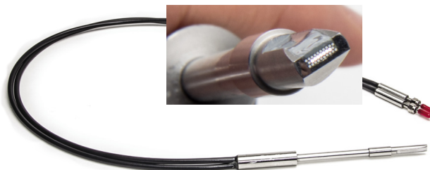
Single emission probe (WPI #94650) for direct sensing of Ca^{2+} via indicator dye Fura-8
